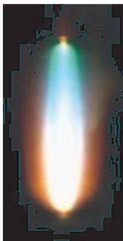
**Figure 7.1:** Colour separation in a metal-halide lamp burner. The lamp is burned vertically upright. See figure 1.1 for full colour.
