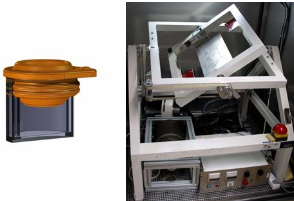
Figure 2. At left a graphical cross section of a polystyrene culture dish used in this study with silicone closing cap securing the insert snug into the well of a 12 wells plate and providing an air bubble free environment. On the right the Random Positioning Machine (RPM) used in this study to simulate weightlessness. The RPM is equipped with a computerised temperature and motor control. The control samples are secured on one of the machine support struts, while experimental samples are placed on the inner frame of the clinostat.
