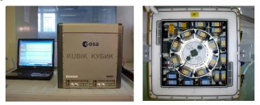
**Figure 1.** Plungerbox. A. schematic representation of an automated tissue culture module (20x40x80 mm) made of a single block of polysulphone (PSU) as it was developed by the Centre for Concepts in Mechatronics (CCM; diagram courtesy of Dr. van Loon; HW, waste or sample holder; PL, plunger; FR, fluid reservoir). B. Plunger box unit with nitric oxide (NO) sensor (arrow). C. KUBIK incubator and centrifuge facility. Pictures courtesy of Centre for Concepts in Mechatronics (CCM).
